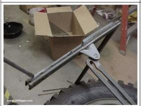
Now the pesky rubber seal. This was hard and frail around my frame. I broke the edges off all the way around, and shot some penetrating oil around the frame. I then got a small screwdriver and pried the rubber seal out.
