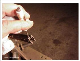
Don't do this!!! I got that little screwdriver out and ended up jamming it into my thumb (notice the wrapped thumb. I ended up using a wire brush on my grinder and just shaved the rubber out. Piece of cake.
