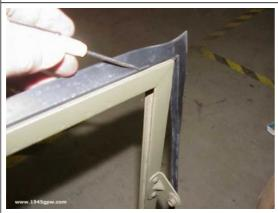
It turns out, the easiest method I found was to use a small screwdriver to insert the rubber seal. Stretch the seal from corner to corner and tilt one side of the edge of the seal into the grove. Use your small screw driver to push in about an inch on one corner then, do the same on the other side. The seal will now be in place for you to push the seal into the slot.
