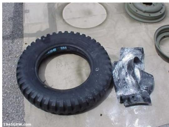
Once the rims have dried completely after a couple days you are ready to install the Flaps, Tubes and Tires. For the first tire install, place the tube in the tire and fill slightly with air. Not much, just enough air to keep the shape up.
