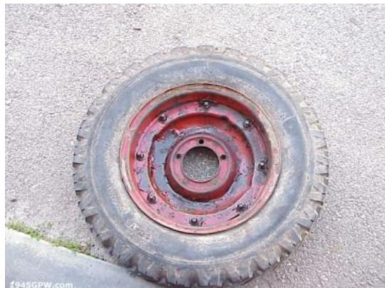
Once the bead is broken on the tire you need to separate the rims. The nuts are usually rusted on tight. Soak them with penetrating oil. This may take a couple days of soaking each nut on the backside. After each attempt of soaking, you can try and unscrew the nuts.
