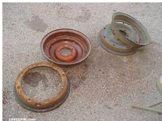
Now the rims are ready for blasting. The rust just peels off with a touch of the hand and should clean up very well.
