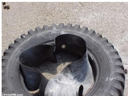
TIP: This part can be a little messy and frustrating. Pre-install the flap on the tube but add baby powder to the flapp so it will slide around. Rubber on rubber does not slide well. Place the stem opening on the tube opening and pull the stem through the flap stem hole.
