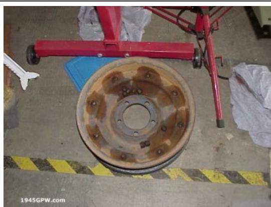
Assuming that you were able to remove the nuts from the back side, you can now take a screw drive and try and separate the rims. It may need soaking between the rim seam as well. This should come apart fairly easily.
