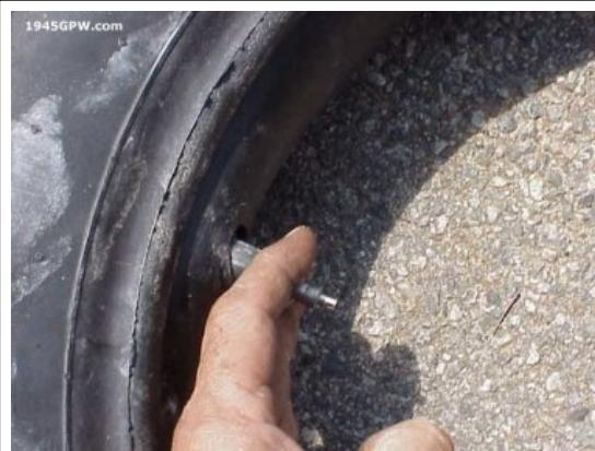
Stuff the flap into the tire around the tube. Pull the stem out, and add a couple of WASHERS around the stem and place the stem cap on the stem so you can pull the stem out. Note: the stem will want to retreat like a turtle pulling his head into his shell.
