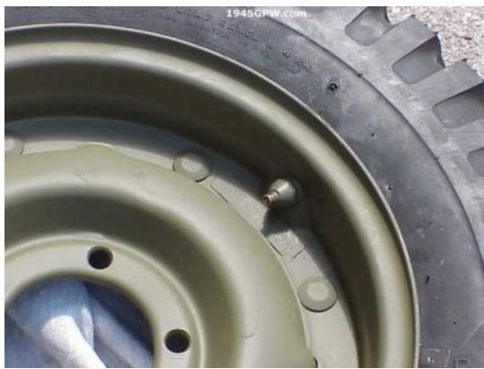
Next, line up the stem with the tube and rim half. Undo the stem cap with washers and pull stem through rim and add screw on the valve stem extender on outside of rim. Then add the other half of rim making sure you don't pinch the flap or tube.
