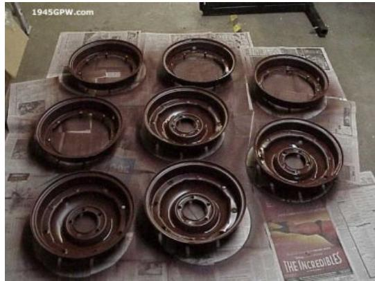
Primering is complete, both sides, making sure you have a good coat of protection especially where the rims will come together.
