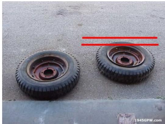
Cleaning up combat rims is a little time consuming. You can do this, while working on another stage of your restore because it is an isolated task. The first thing to do is break the bead on the existing tires. Remove the valve stem to let the air out of tire. Then take another vehicle and run over the tire as shown in read lines.
