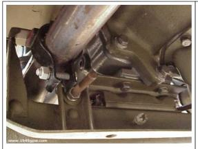
Tighten the bolt so it is snug but not tight. The purpose of this cable is to stop the engine from going forward driving the fan into the radiator or some other damage. Without this cable, a drop in a forward position can drive the engine forward and cause significant damage.
