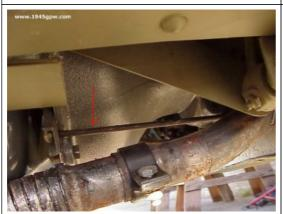
Here you see in the photo that one end of the cable is a knob that will slide through the engine back plate and extend back to the crossmember that the transmission is resting on.
