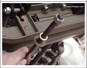
Here you see the back of the stay cable which is tightened by a bolt. You want to slide it through the bracket on the crossmember shown with an arrow.
