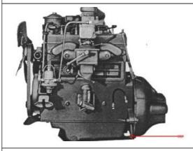
The Engine Stay cable tends to be a missing piece on most unrestored, farm found jeeps. If you are restoring your WWII Jeep to drive around regularly, you should make sure that you include this valuable item. In the photo, you see that the cable connects to the Engine rear plate.
