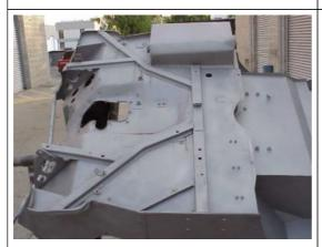
In addition, the clean surface allows you to inspect the metal for weaknesses. It was very easy to spot areas that I needed to replace due to weakness from rust or pitting. The surface is ready for welding as well!
