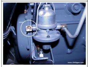
Before you install your fuel pump look at what is going to get in the way first. The top brass fitting MUST be installed on your pump first, because you will not have any room to spin it once your pump is tighted down. The other issue is how to reach the bolt on the left that holds the pump to the block.
