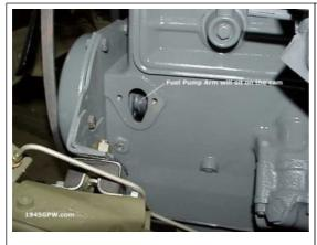
(Tip from Pete Silfven) Before installing, rotate the engine so the fuel pump cam is all the way down. Using a 1/4 inch drive extension and a short 1/2 inch socket, insert the front bolt into the pump. Then install the whole thing on the engine using the extension and socket to start the front bolt.
