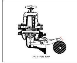
For reference, the fuel pump arm will sit on the cam shaft, and as the cam shaft rotates the lever on the pump will go up and down thus pumping the fuel.
