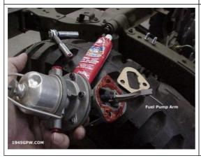
(Optional) If you want a good seal, then you can add a little sealer around the gasket prior to installing. Here you see to much sealer, smear this around the gasket with your finger and remove excess.
