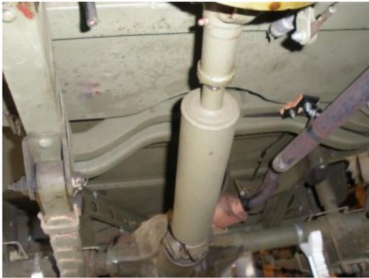
Done! your rear propeller shaft is installed. Place your gears into the neutral position and spin the wheels and review the axles moving and u joints spinning correctly.
