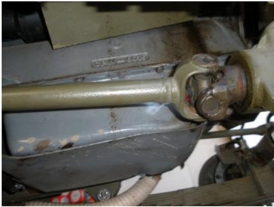
Complete the install by moving to the otherside of your propeller shaft and repeat the steps for installing the u-bolts.
