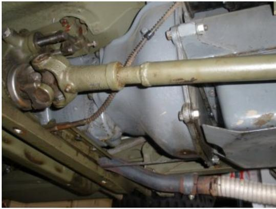
Line up the flange yolk on the transfer case and loosen the U Bolts, attach around the u-joint and tighten.
