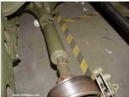
Like the front shaft install, stretch or compress the propeller shaft to line up with the rear axle. Here you see the rear drive shaft as the "fat" model. We are working on a late model GPW, your rear propeller shaft maybe the "thin" version.
