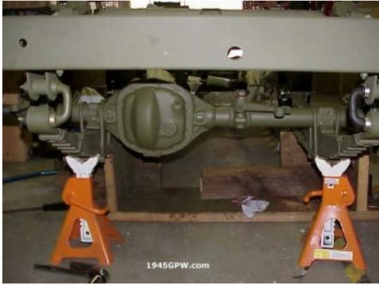
Installing propeller shafts is not a difficult job. To start with, make sure your jeep is off the ground and the transmission. Place your transfer case gears to engage in 4W high or low, otherwise when you try and tighten your u-bolts the axle will want to spin.
