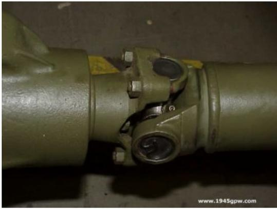
Loosen the U bolts on the rear axle and align the u-joint into place. Tighten the U bolts into place.
