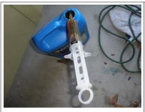
Now, use your SAE 90 wt oil and a device to pour into the top of the steering plug hole. Here you see a very inexpensive surenge that will allow us to insert the oil into the housing easily and without mess.
