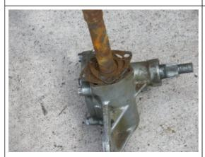
Loosen the upper housing clamp and pull up the tube, then unscrew the 3 bolts holding the upper housing cover. You should be able to pull the tube up off the steering column.
