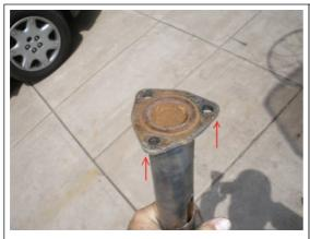
With a rubber hammer, tap the upper housing cover off the tube. This should separate easily.
