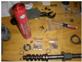
Now, prepare to install the main worm gear shaft. Here you see we will prepare with the new balls, rings, cups, and have some grease ready.
