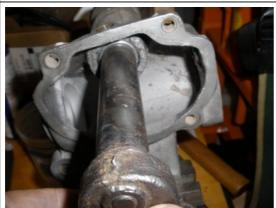
After you have the bushings pressed in, test the fit with the shaft.
