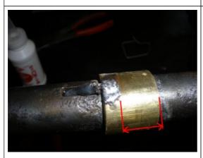
Solder is a nice fit with plenty of room for the brush to ride along the bottom half of the fitting.
