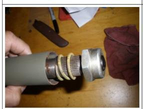
Now install the steering wheel spring and the steering nut with horn button so that the wire and contact do not get bent up.
