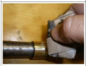
Next prepare the soldering area on the bushing by sanding the section that you will solder on. Note: the top of the bushing is where the contact will ride on the bushing from the steering column.
