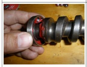
Start by installing the balls in the lower cup. Place some grease in the cup because the small ball bearings will slip out, and the grease will cause them to stick. Start with adding a couple balls, then press the cup on and put the rest of the balls in. Note: you can prep with all the balls because it will not fit over the retaineron the worm drive.
