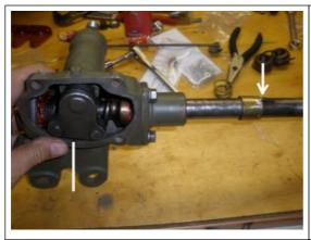
The sector shaft should push all the way through and line the teeth up on the worm shaft in the center. Here you see the contact ring is lined up in the middle of the shaft. If you have issues, you will want this lined up with straight wheels later.
