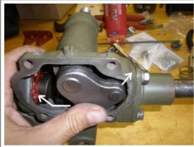
One the sector shaft is in, turn the main core shaft and feel the sector shaft fit with the worm gear and verify that it is lined up in the middle where the contact wire is facing upward as mentioned before.
