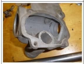
Blast the housing and clean out all the area where the new cups and bushings will be replaced.
