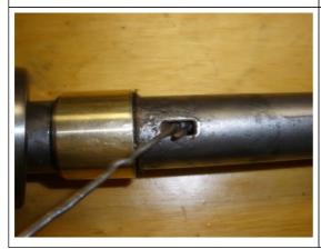
When you pull the wire back and you get to the opening in the shaft it is going to be very tight. You need to twist the pull wire while pulling about 90 degrees before the wire will fit through the opening.
