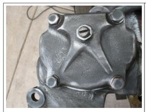
Here you see the side cover is cleaned off so we can prepare to remove it. Ford Owners Note the F mark on the side cover.
