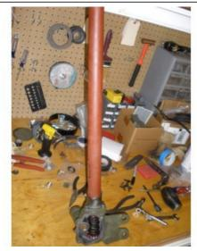
Install the main tube over the main shaft. Here, check two things. First the turning of the main shaft that there is no drag, and second look to see if you contact arear for the orn is linged up. Note the position of the contact area hole. Should be pointing upward for the connection to the horn after you install the steering.
