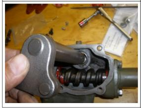
Now, insert the new sector shaft into the housing with the new bushings. In this case, the fit was to tight for the second bushing, so we needed to hone it out a bit to get it to fit through.
