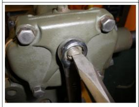
With the cover bolted on, rotate the cover screw clockwise while turning the main shaft. Turn until you feel a slight drag on the sector shaft while turning. Back off just a bit, and tighten the nut around the cover plate screw. Test the main shaft moving from one end to the other.
