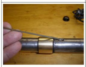
Run the wire down the steering shaft to top end. There we will hook it up and pull it back through.
