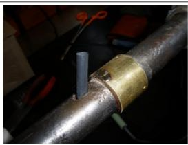
\*optional\* here we put a little extra protection on the wire with a little heat shrink wrap. When the wire is being moved around with steering, this will protect it around the hole it comes through. In addition, we prep the bushing with a little solder prior to bringing the wire down.
