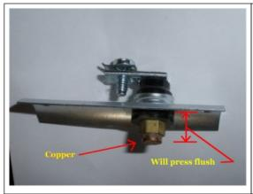
Tip: Buy a quality contact brush! Here you see a quality contact brush that will compress to be flush, and the contact area is copper (like the ring). The repo contract brush above is garbage compared to this one.
