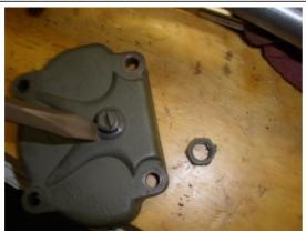
Before you replace the cover plate on the housing, you want to loosen up the screw on the housing plate. This screw keeps the sector shaft from pushing itself out of position when the worm shaft is moving. If it is on to tight, the sector shaft will not move.
