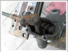
By rotating the steering column, you will see the lever shaft start to force itself upward. You can pull this out with your hand, or wedge a screwdriver in and finish bringing it out.
