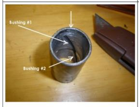
Take a look at your replacement bushings. From the replacement kit, you will see the short and long bushing together. Observe the grove in the middle. This is for lubrication flow on the shaft. The longer bushing grove stops before the edge so that the lubrication does not make it to the seal and leak.
